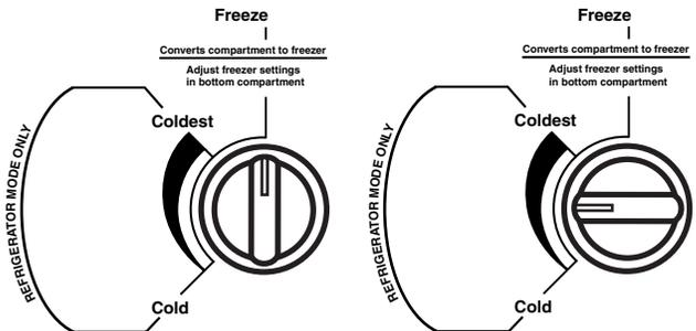
**IMPORTANT:** If the control is set between FREEZE and COLDEST settings, the upper compartment may not operate in the desired mode. The control should be set all the way to FREEZE to function properly as a freezer, or in the range between COLD and COLDEST to function properly as a refrigerator.
